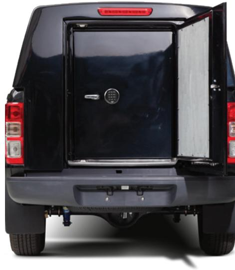
Discreet security cash box manufactured from steel frame structure covered with aluminum sheeting of 2mm thickness, mesh weave and heat insulation for fire protection.
